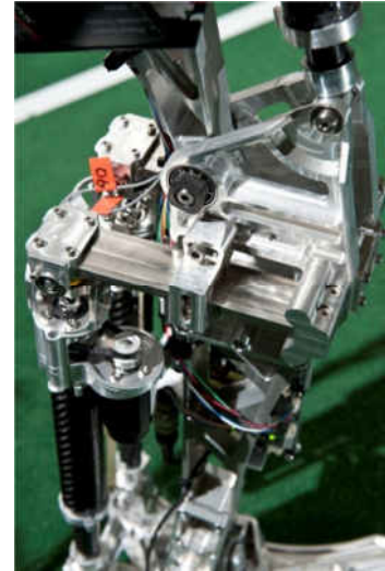
Figure 4: Titanium compliant members in series with the two ankle actuators.
