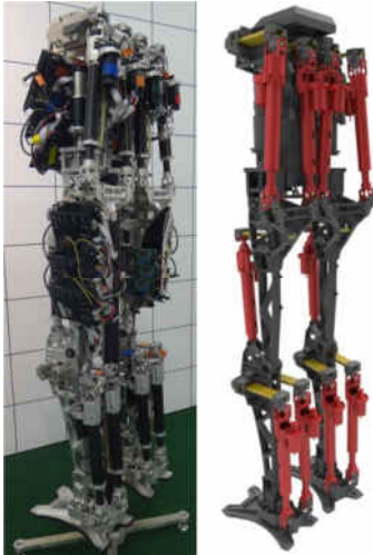
Figure 3: Linear actuators shown in red against SAFFiR's structure. Compliant beams shown in yellow.
