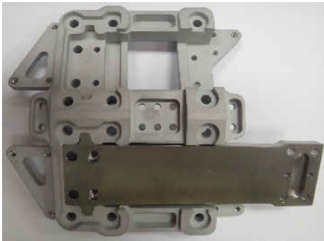
Figure 10: Compliant spring mounted in the standard interface
