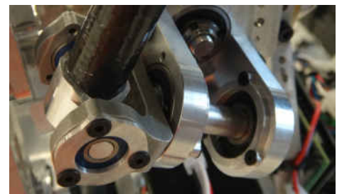
Figure 13: Universal joint connecting hip actuator to the coxa
