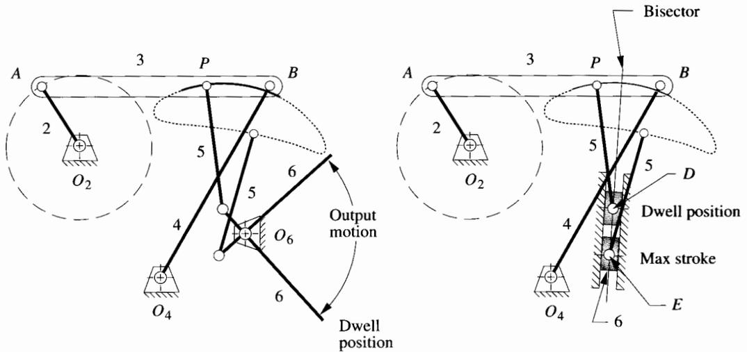
(c) Completed sixbar single-dwell linkage with rocker output option
