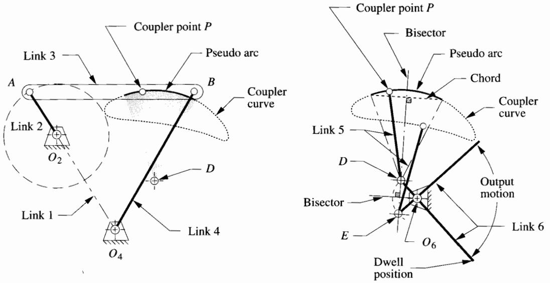
(a) Chosen fourbar crank-rocker with pseudo-arc section for  $60^\circ$  of link 2 rotation
